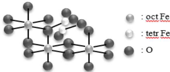
Gambar II.1 Struktur Kristal \text{Fe}_3\text{O}_4 (Maylani, 2015)
