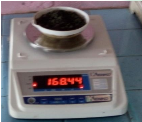
Penimbangan cawan porselin + sampel aspal
