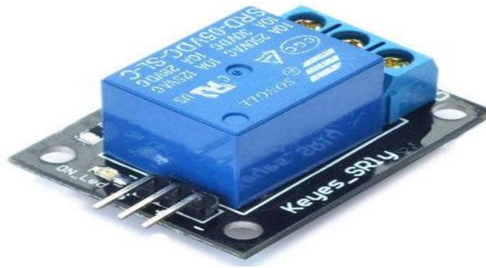
Gambar II. 8. Relay 1 Channel
