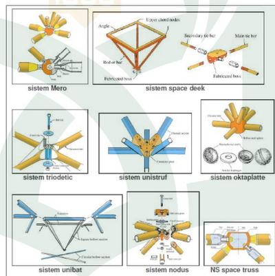
Gambar III.27. Sistem joint
