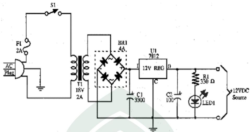
Gambar IV.5 Rangkaian Power Supply
