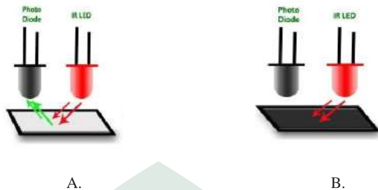
Gambar II.5. Cara Kerja Sensor Photodiode
