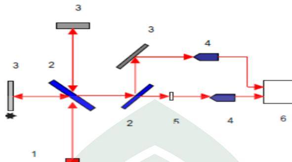
**Gambar 2.3** Skema Alat FTIR (*Fourier Transform Infra Red*)
