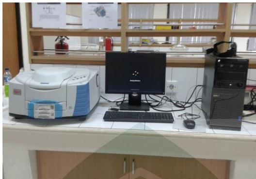
**Gambar 2.2** FTIR(*Fourier Transform Infra Red*)
