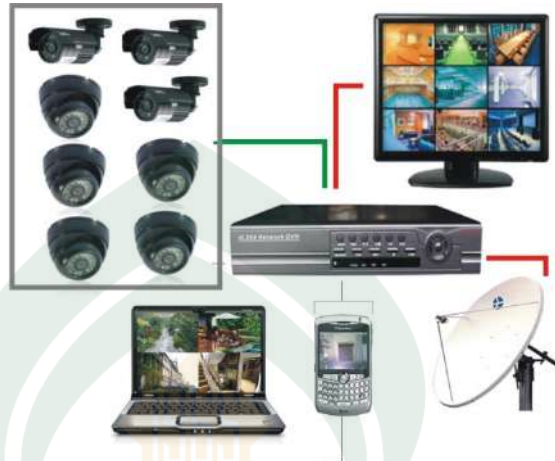
Gambar IV.28. Skema Sistem CCTV Sumber : http://wijanarko-aficom.blogspot.com/2016
