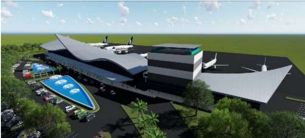
Fig. 10. Application of metal sheet roof material
