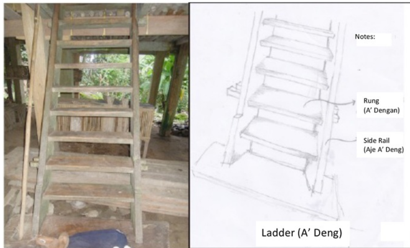
Figure 3 : Ladder detail for Karampuang traditional house
