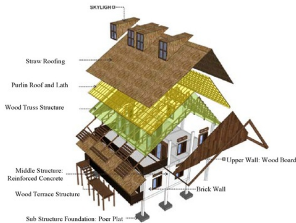
Figure 9. Terraced house building structure
