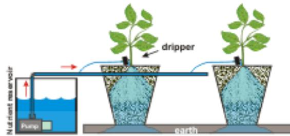
Fig 1.5a Run-to-waste system (Basic layout): Nutrient run-off drains directly onto the ground.
