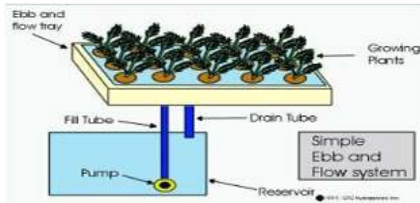
**Gambar 2.6** Hidroponik *ebb and flow system* (Natalia, 2017).
