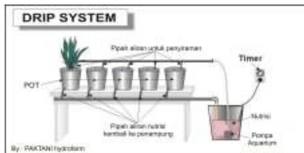
**Gambar 2.5** Hidroponik *drip irrigation* (Natalia, 2017).
