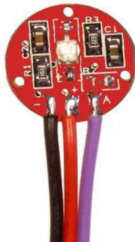
GambarII.7 Pulsa sensor tampak belakang Sumber: Joel. 2012. Anatomy of The DIY Heart Rate Monitor .
