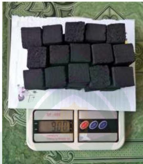
Gambar 3.6: Mengukur briket
