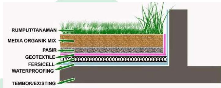
Gambar II.4 Lapisan Sistem Roof Garden
