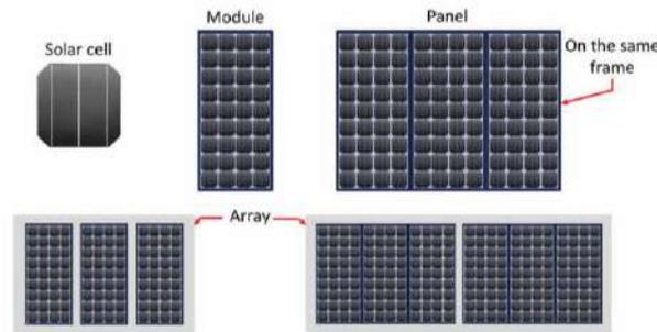
Gambar II.6 Diagram Hubungan Sel Surya, Modul, Panel & Array
