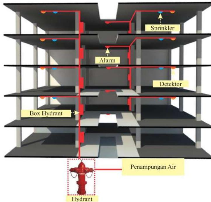
Gambar IV. 7 Sistem Fire Protection
