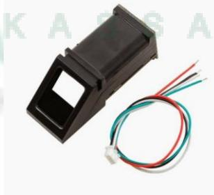
**Gambar II.4. Sensor Fingerprint**
