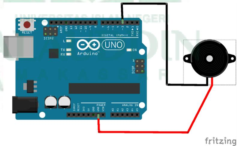
Gambar IV.7 Rangkaian Buzzer
