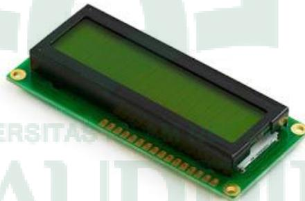
**Gambar II.6. LCD (Liquid Crystal Display)**
