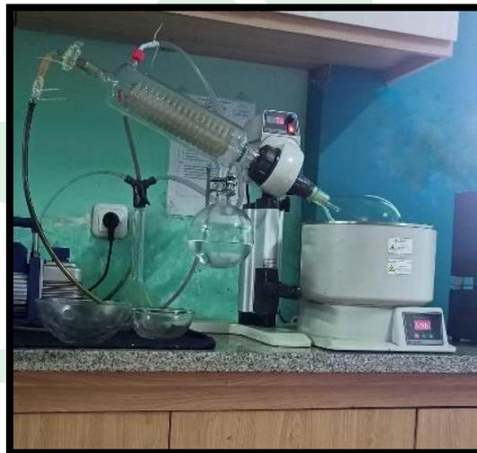
**Gambar 6.** Proses Rotary Evaporator Ekstrak Bajakah Tampala
