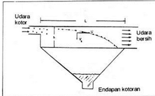
**Gambar 10.3:** Alat Pengendap Sistem Gravitasi (Wardhana, 2001)
