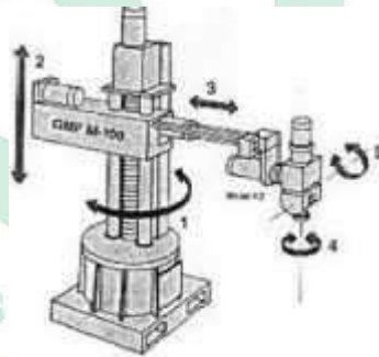
Gambar II.2 Cylindrical Coordinated Robot (Sumber : www.societyofrobots.com )
