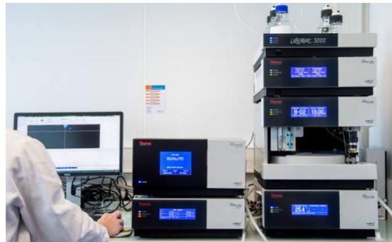
Gambar 2.3. Alat HPLC ( high performance liquid chromatography )
