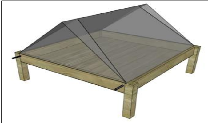
Gambar VII.4: Solar Still Double Slope (prisma)
