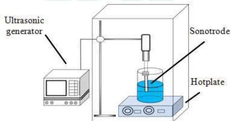
Gambar 3. Alat *Ultrasound-Assisted Extraction* (Lully, 2016).
