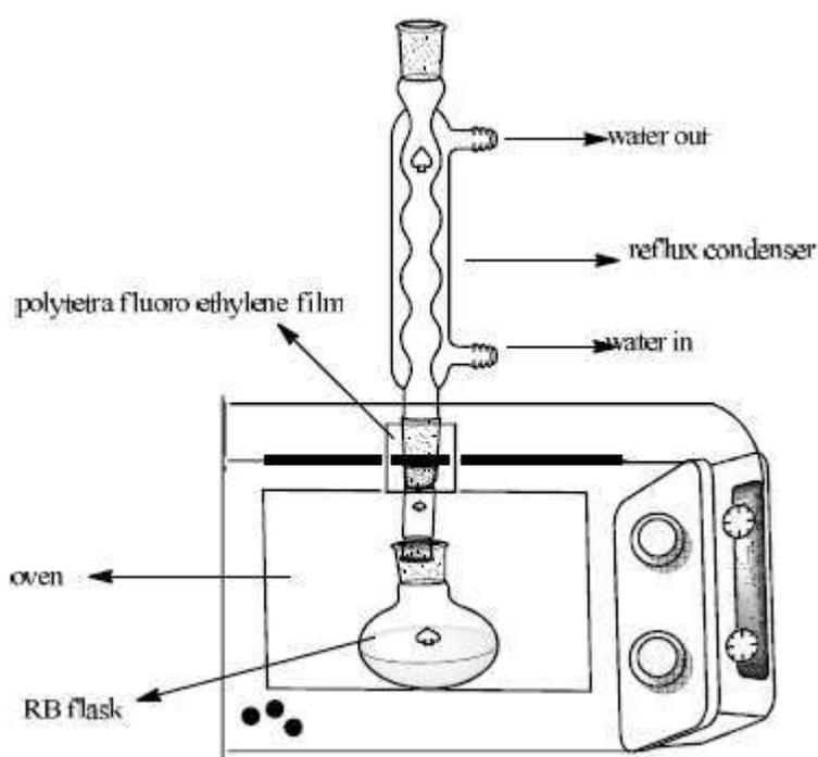
Gambar 4. *Reaktor Microwave-Assisted Extraction (MAE)* (Lully, 2016).
