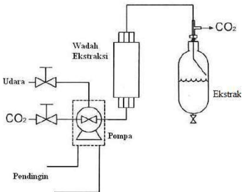
Gambar 5. *Supercritical Fluid Extraction (SFE)* (Lully, 2016).
