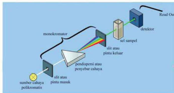
Gambar 8. Diagram alat spektrometer UV-Vis (single beam)
