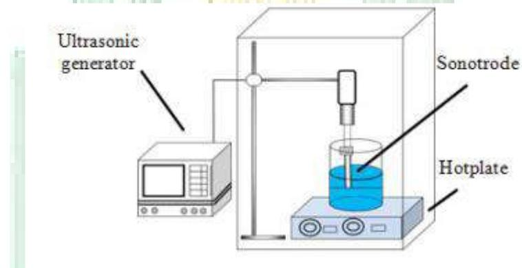
**Gambar 6.** Alat Ultrasound-Assisted Extraction (Julianto, 2019:24).
