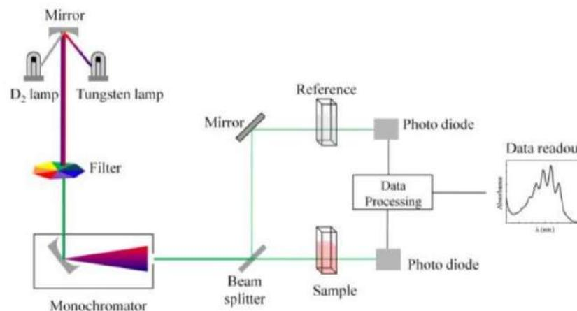
**Gambar 7. Prinsip Kerja Spektrofotometri Uv-Vis (Moch. Amin Thohari,2015)**
