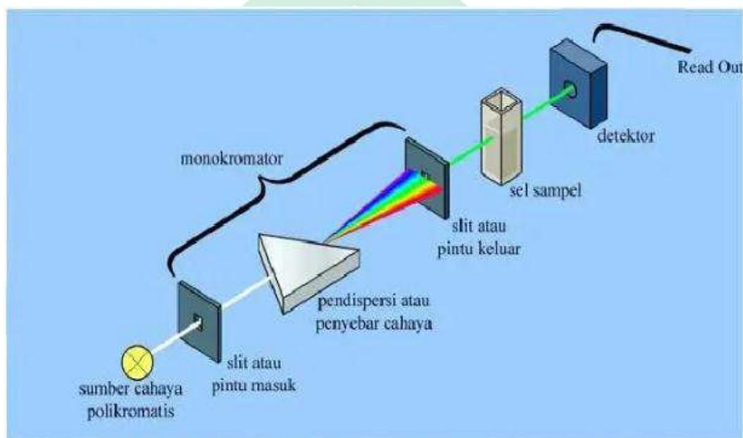
**Gambar 8.** Spektrofotometri UV-Vis Single-beam
