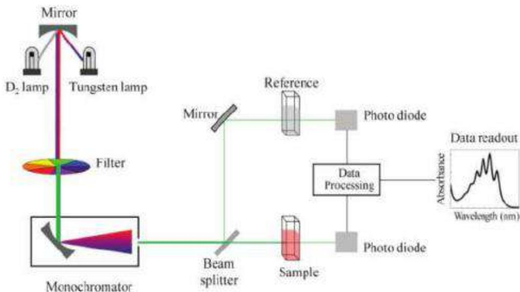
**Gambar 9.** Skema Spektrofotometri UV-Vis Double-beam
