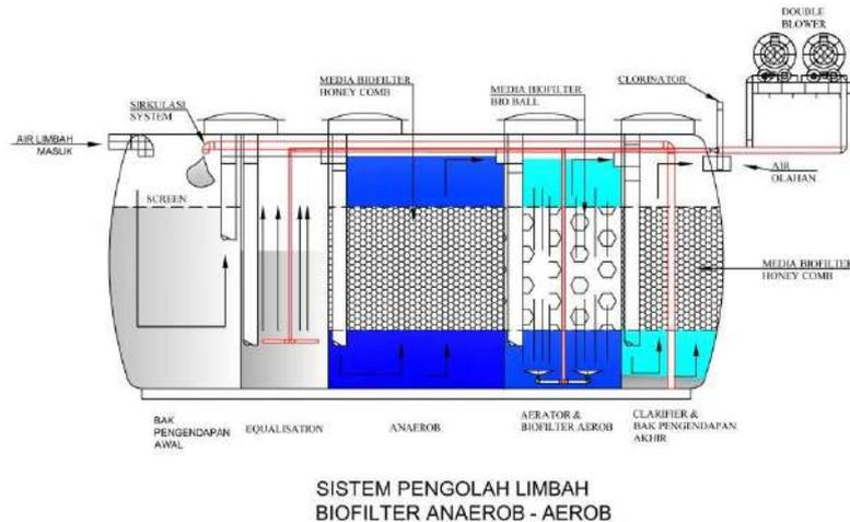
Gambar III.36 Skema IPAL Biofilter
