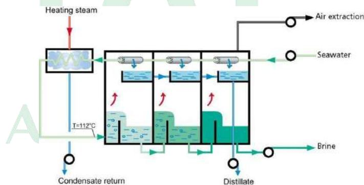
Gambar III.33 Prinsip *Multi Stage Flash (MSF) Evaporator*
