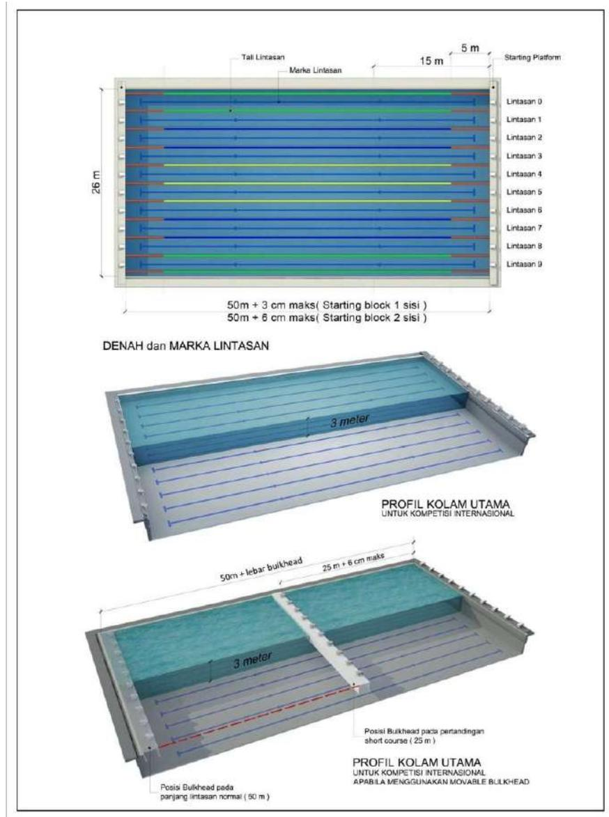
Gambar II.1 Denah Kolam Utama 10 Lintasan
