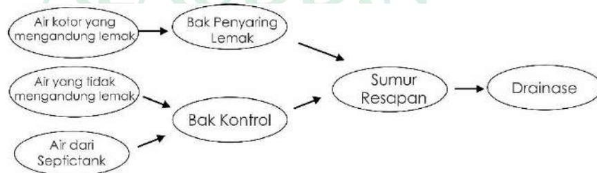
Gambar III.35 Skema Sistem Air Kotor
