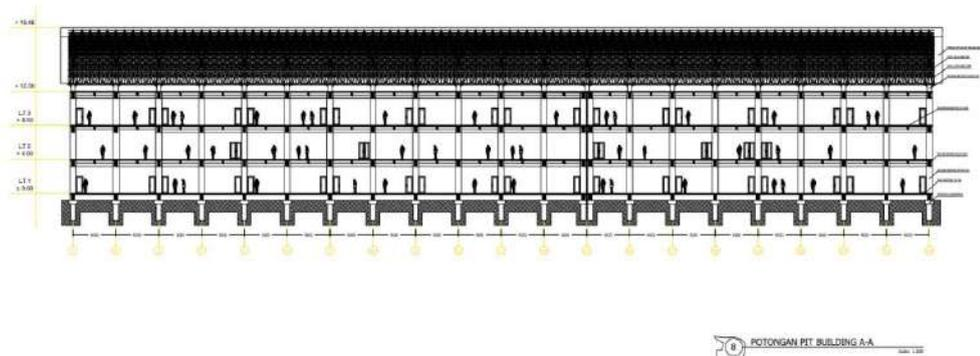
Gambar VI.8 Potongan A-A Bangunan Pit Building
