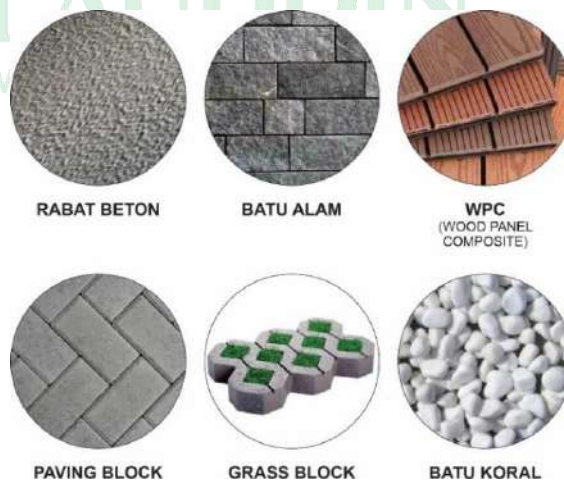
Gambar III. 47. Material Hardscape Sumber : (Olah Data, 2023)
