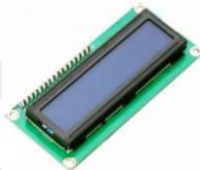
Gambar II.17. LCD (Liquid Crystal Display). (Sumber : https://probots.co.in/16-x-2-lcd ).
