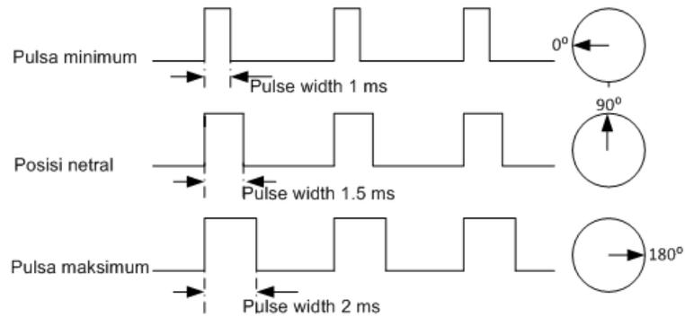
**Gambar II . 8** prinsip kerja *Motor Servo* (google,2016)
