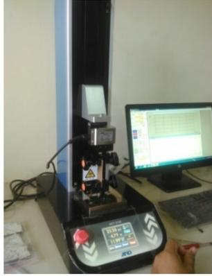
**Gambar 2.8** *Universal Testing Machine (UTM)*
