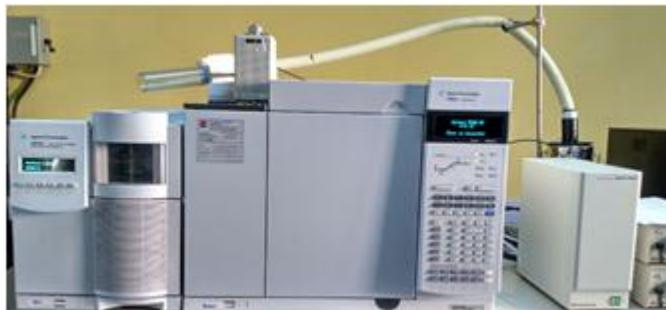
**Gambar 2.9** Spektrofotometer *Gas Chromatography–Mass Spectrometry* (GC-MS)
