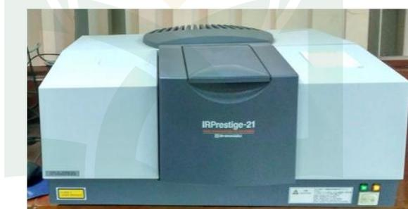
**Gambar 2.8 Spektrofotometer *Infrared* (IR)**
