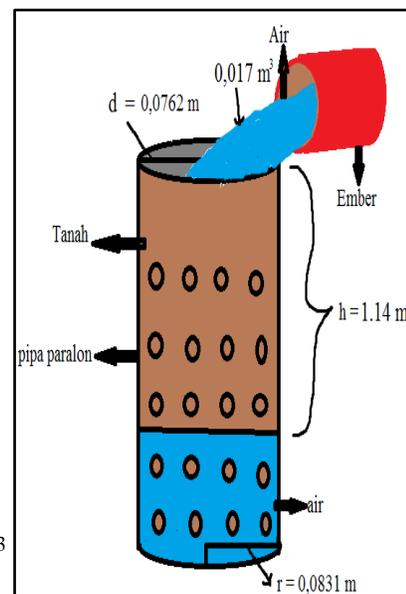
Gambar 4.1: Model pipa biopori
