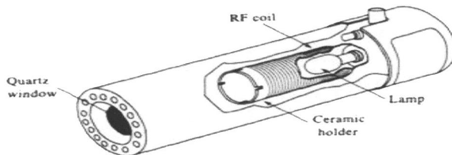
Gambar 4. Electrodelles Discharge lamps
