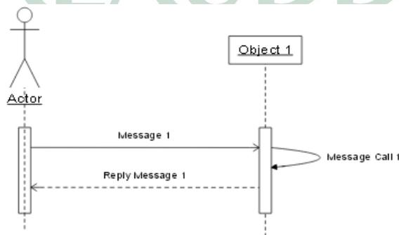
Gambar II. 1. Model *Sequence Diagram* (Munawar, 2005).
