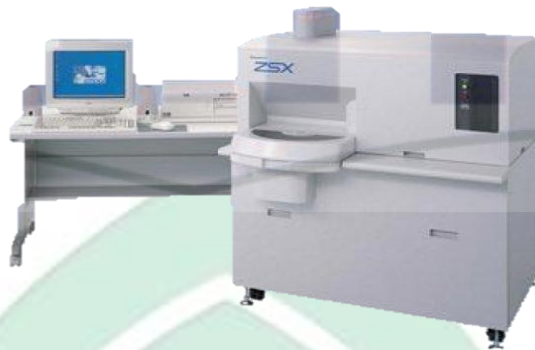
Gambar 2.7 Instrumen X-Ray Fluoresence (Sumber: Krisnawan, 2009)
