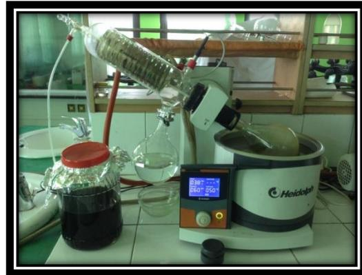
**Gambar 2.** Proses rotary evaporator
